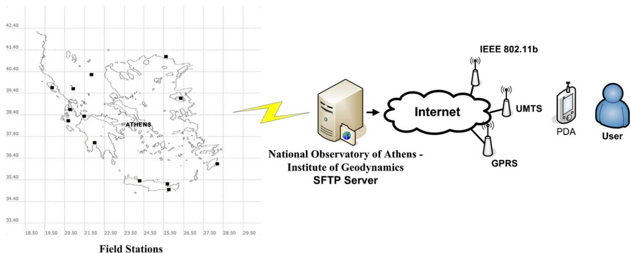
**Fig. 1.** Schematic representation of flow of EM data from field stations to NOIG SFTP server, then distributed via different transfer protocols to PDAs and users.
