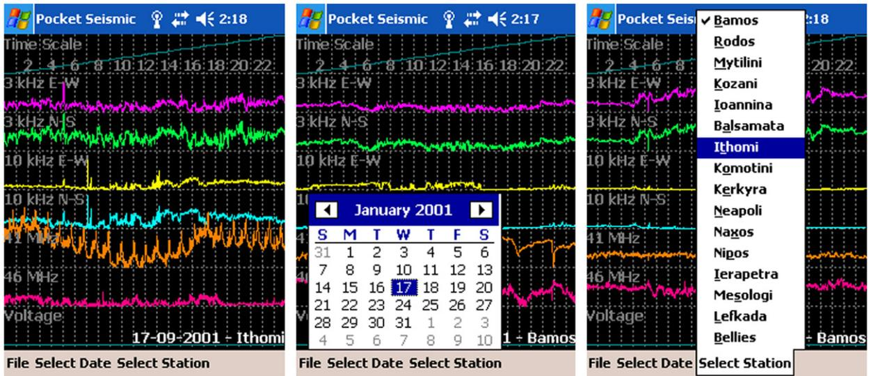
**Fig. 2.** Screenshots of the EM signal display application user interface on a PDA device. (a) Overview of developed EM signal interface. (b) Interactive calendar to allow dynamic acquisition of different EM signal traces for different time periods. (c) Dynamic selection of field station name allows retrieval of EM signal data from different field stations via NOAA SFTP server.
