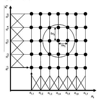
**Fig. 1b.** Two dimensional example: Non-symmetric fuzzy partitioning into seven fuzzy sets for  $x_1$  and five fuzzy sets for  $x_2$ .
