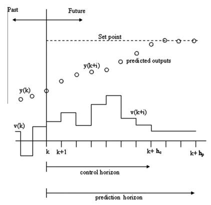
Fig. 2. A graphical representation of the MPC methodology.
