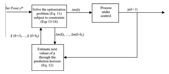
Fig. 3. Integration of RBF model and MPC methodology.
